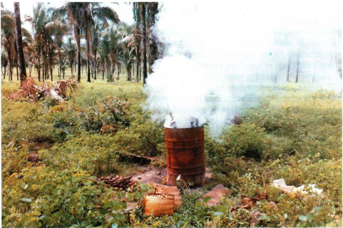
Crude process of making charcoal from babassu shell. (Photo: G. Blaak)
