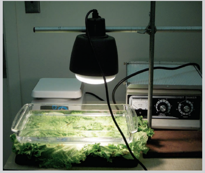
Figure 3. Our apparatus using lettuce leaves as a far-red light filter. Green leaf lettuce was used in this experiment. We have also successfully used red leaf and iceberg lettuce as well as collard greens as a far-red light filter.
